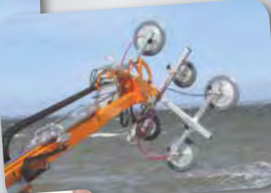
The Smartlift has side shift for exact adjustment of the window
